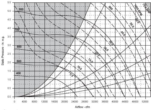
Figure 67: RAH 077C, SWSI fan, 49" airfoil
