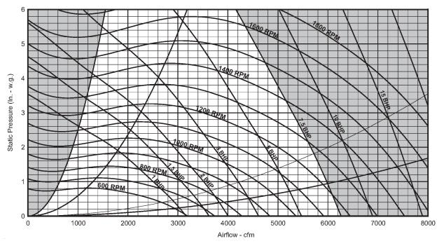
Figure 46: RDS 708B supply fan, 15"×6" forward curved fan
