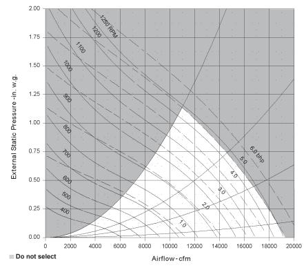
Figure 69: RAH 047C and 077C (2) 36" propeller exhaust fan
