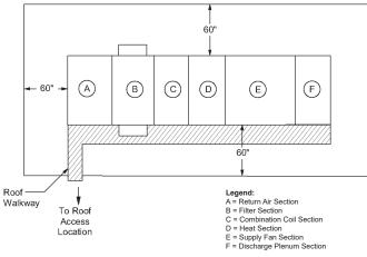
Figure 118: Service clearances—RDS 800C and 802C
