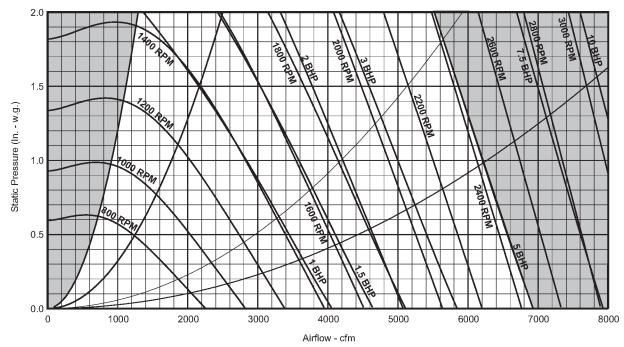
Figure 74: RDS 708B 16" airfoil fan with vanes
