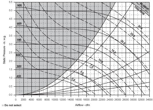
Figure 65: RAH 047C, SWSI fan, 44" airfoil
