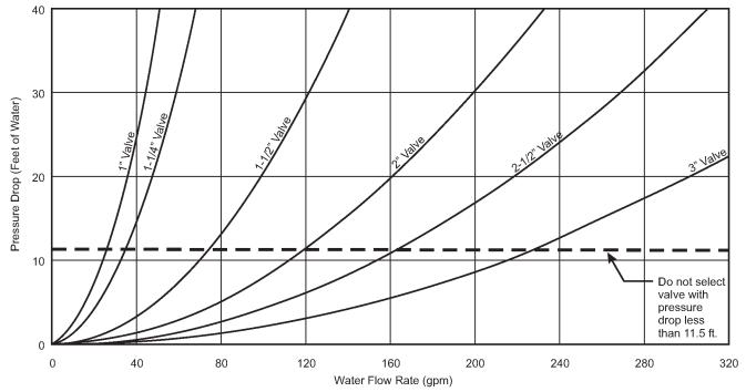
Figure 45: Hot water valve piping pressure drop
