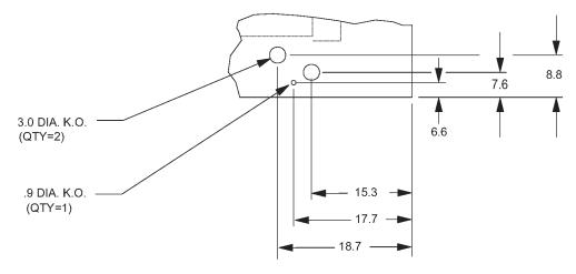
Note: 0.9 diameter and 3.0 diameter knockouts are electrical enterance locations on the unit only.
