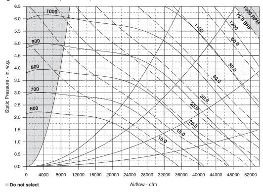
Figure 63: RAH 077C, DWDI fan, 40" airfoil
