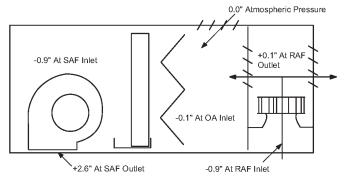
Exhaust fans are very different than return fans and cannot maintain proper building pressure and ventilation control as return ESP increases.
