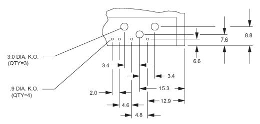
Figure 115: Discharge plenum power and control wiring entrance detail
