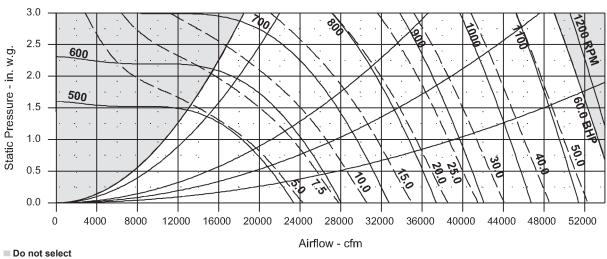
Figure 79: RAH 077C SWSI fan, 44" airfoil
