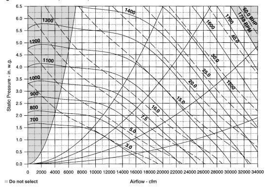
Figure 59: RAH 047C, DWDI fan, 30" airfoil
