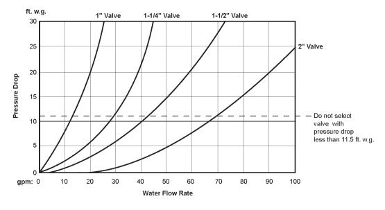
Figure 39: Unit chilled water valve and piping pressure drop
