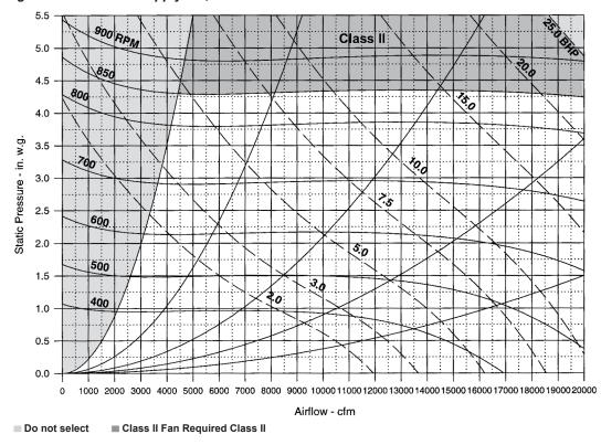
Figure 55: RDS 802C supply fan, 24" forward curved fan
