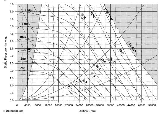
Figure 61: RAH 077C DWDI fan, 33" airfoil
